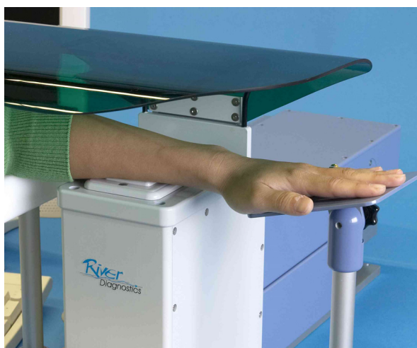
Figure 1. The River Diagnostics model 3510 depth-scanning skin analysis system can non-invasively analyze molecular concentration profiles in the skin.
